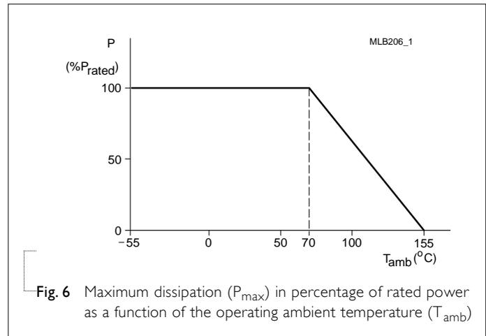
Fig. 6 Maximum dissipation ( $P_{max}$ ) in percentage of rated power as a function of the operating ambient temperature ( $T_{amb}$ )
